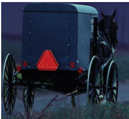
Animal-drawn vehicle displaying SMV emblem only, Photo credit: Pennsylvania Department of Transportation
